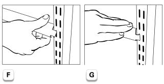
Identify the top of the back stop bar as shown in Fig F.
