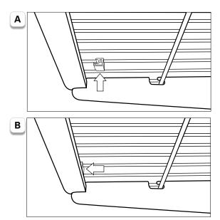
The top of the clip features a groove that accommodates one shelf wire. (FigureA) Once it's attached to the underside of a shelf wire, slide it all the way to the front of the shelf and into the opening of the fascia for a secure hold. (Figure B).
